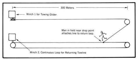
Bob Denny of Silver Spring, Maryland came up with an easy retrieving system for Glider Towlines. The trick is a continuous loop on one winch. Let your fingers do the walking. See text.
