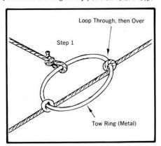
Towline now self-tightens itself upon the ring, signal starts the distant winch and the line is retrieved with a minimum of time and footwork.
