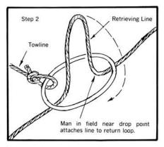
First pull a slack loop in the line as in Step 1. Next, flip it over the tow ring. This system lets you attach the ring at any point on return loop.
