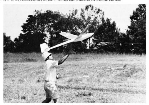
The winner! Otto Heithecker accomplished an almost unbelievable performance at June 4 D.C.R.C. Soaring meet. Four max flights of 10 minutes were landed inside the spot within a total of seven seconds error. A total score of 2593 out of 2600! He used a Cirrus wing scaled up to 12 feet in span on a home design fuselage and tail. A capable aircraft. Photos by Bob Denny.
