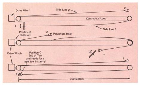
A really clever idea for a Winch system by Bob Denny. It's ready to go the instant the previous glider is released. The above diagram represents one winch in three separate stages of a tow. (Not three winches.) All is described in text. Great for big R/C Soaring meets, clubs, etc.
